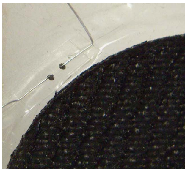
Fig. 2. Photograph of a MEA with the DHE unit attached just outside the gas diffusion electrodes. The gap between the ends of the two Pt wires is ca. 1 mm.
